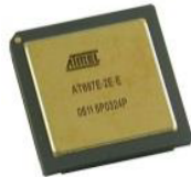
AT697 LEON2FT (Atmel, 180nm)
