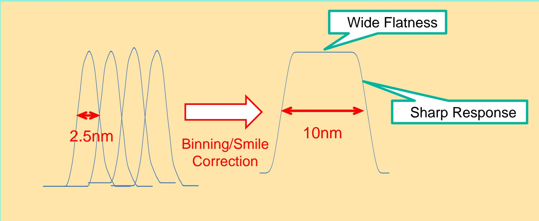
data binning in spectral direction
