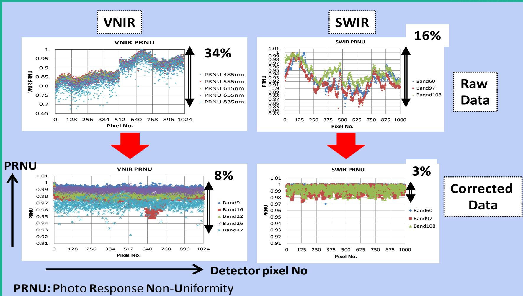
(\*) Based on the data of Evaluation Model of the sensor
