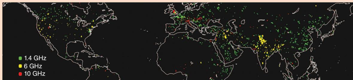
**FIGURE 1.** Map showing RFI detected at three different frequencies: RFI at 1.4 GHz as observed by the Aquarius radiometers during December 2011, RFI at 6 and 10 GHz as observed by AMSR-E during December 2010.
