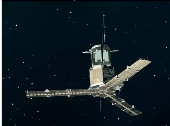
MIRAS consists of a central structure (hub) and 3 deployable arms, each of which has 3 segments.
