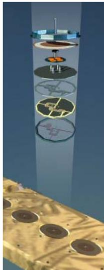
The LICEF antenna provides best performance in terms of gain, bandwidth and differentiation of horizontal and vertical polarisation components of incoming microwaves.
