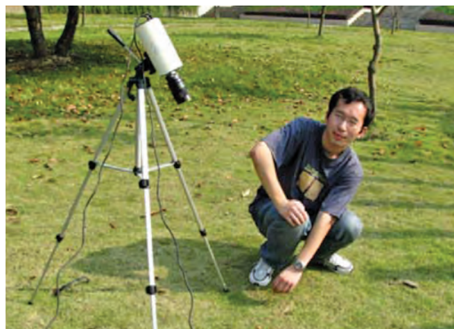
Figure 1. Obtaining near scene hyperspectral images by a CRI camera
