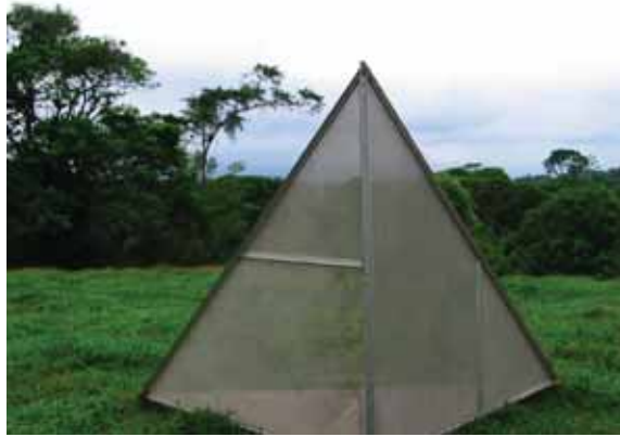
Trihedral reflector deployed in Costa Rica by the author that is similar to the one planned to be built in the GRSS project.
