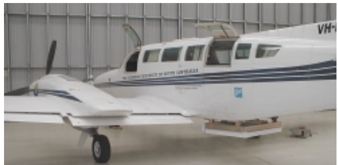
Figure 1. Airborne Research Australia's Cessna 404 with the SLFMR mounted beneath the fuselage. The aircraft is equipped with a general-purpose flight data acquisition system and navigational systems that provide precise environmental and positional data which is merged with passive microwave measurements from the SLFMR.
