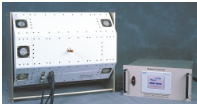
Figure 4. Liquid-cooled 95 GHz cloud radar and stand-alone instrument controller. Fans for optional heat exchanger are mounted on ends of RF unit.
