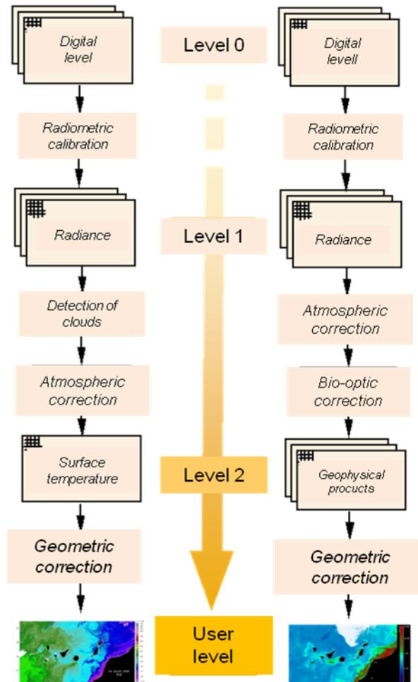
**Fig.1.** - Generic hierarchy of processing levels applied to NOAA-AVHRR data.
