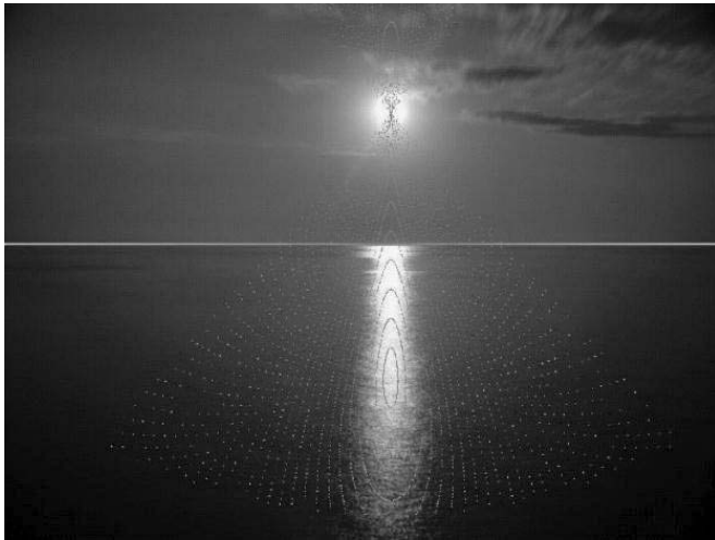
Figure 3. Sun glint over the ocean. The coordinates provide a “tilt-azimuth map”, i.e., for each surface point the facet inclination angles required for the facet to forward the energy towards the camera (receiver). The image intensity as a function of these coordinates can be used to infer the surface roughness. For example, for a rough ocean with large surface slopes, the “glistening zone” will become very large. The use of sun reflections to estimate sea state has a long history (see [Spooner, 1822]).
