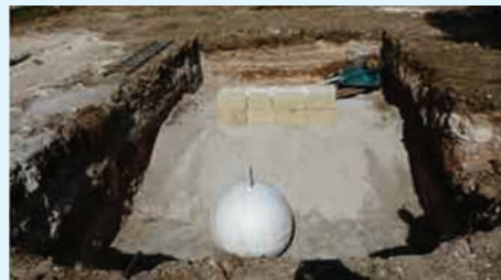
A polystyrene sphere, simulating a cavity, with a tuff wall simulating a foundation
